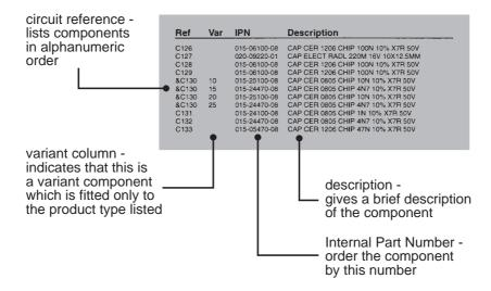
The miscellaneous and mechanical parts are listed in IPN order at the end of the parts list.
